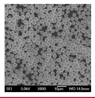
Mono-dispersed Proteomix ionexchange particles enable uniform column packing bed, which improves separation efficiency.
