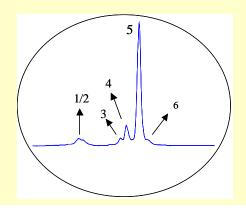
Figure 6 is a typical test chromatogram for a 5  $\mu$ m, Proteomix SAX-NP column for separation of a mixture of ovalbumin and BSA. High resolution and high selectivity of Proteomix SAX-NP phase can well separate the impurities contained in ovalbumin sample, as well as the BSA dimer from BSA.
