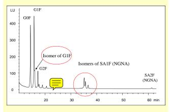
Column: Proteomix SAX-NP5 (5  $\mu$ m, 4.6x150 mm) Mobile phase: A, 2.5% (v/v) acetic acid, 0.5% TEA in H<sub>2</sub>O
