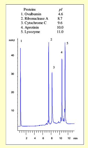
Column: Proteomix SCX-NP3 (3 µm, 4.6x50 mm)
