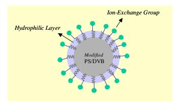
Figure 1. Schematic illustration of the chemical structure of Proteomix ion-exchange phases.
